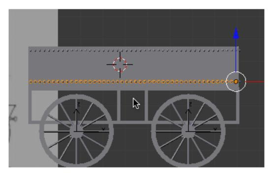
Select both duplicate plates and duplicate rivets and make a duplicate copy for the other side of the car. You will have to rotate them around the X-axis 180 degrees.
