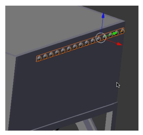
Since these are their own objects we can edit them including the array modifier. Select the plate object. TAB into edit mode and extend the vertices to the edge of the car. Select the rivets object and in the modifier panel increase the count to 18 (or whatever you need to fill up the plate).
