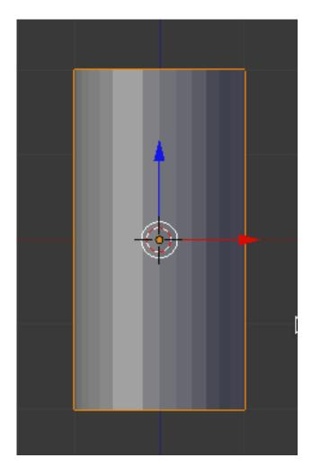
TAB into edit mode. Press CTRL-TAB and select edge select. Box select the center edges of the tube and press the Subdivide 6 times (we need plenty of vertices to model this pipe fitting).
