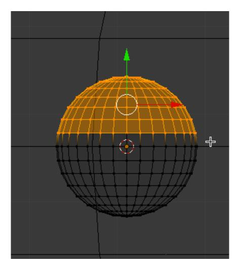
Press the XKEY and delete the vertices. TAB out of edit mode. Select the object and move it down along the Y-axis so that it is just outside of the collar object as shown below.
