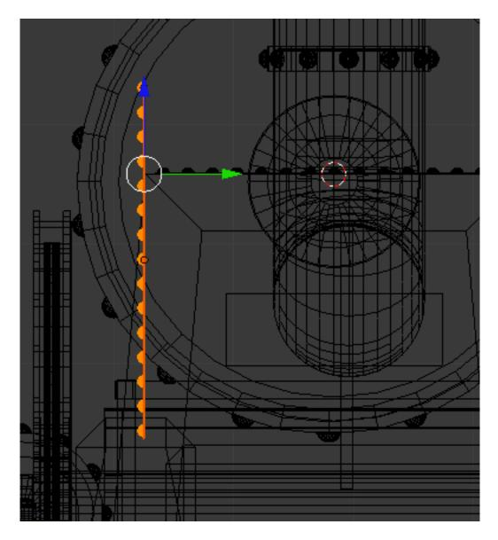
Press the RKEY followed by the XKEY and rotate the objects so they align with the angle of the side of the furnace as shown below.
