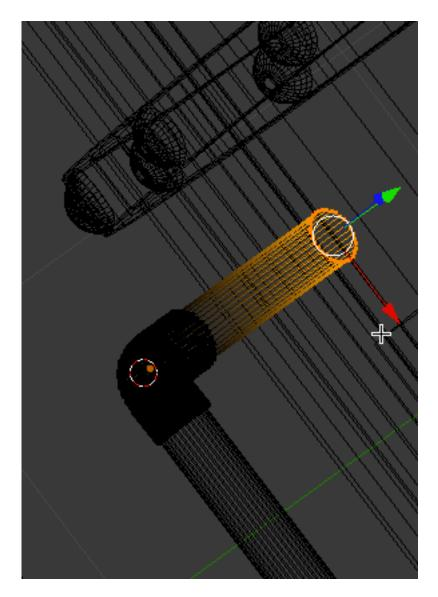
TAB out of edit mode. Select the 2 objects and press CTRL-J and join them together into one object named "Pipe 1".
