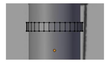
TAB out of edit mode. Press SHIFT-CTRL-ALT-C and select origin to geometry. Name this object "Stack Collar".
