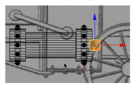
TAB into edit mode and select the left set of vertices and scale them out a bit and then select the right set of vertices and scale them down a bit as shown below.
