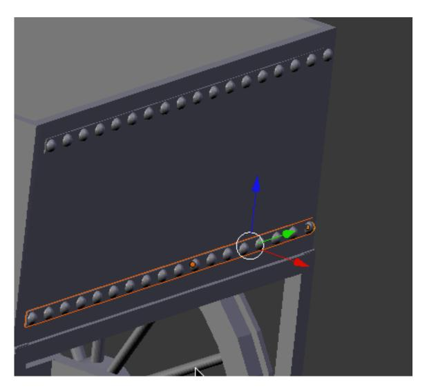
With the duplicate objects still selected, press SHIFT-D and make another copy of the objects and move it out along the Y-axis as shown below.
