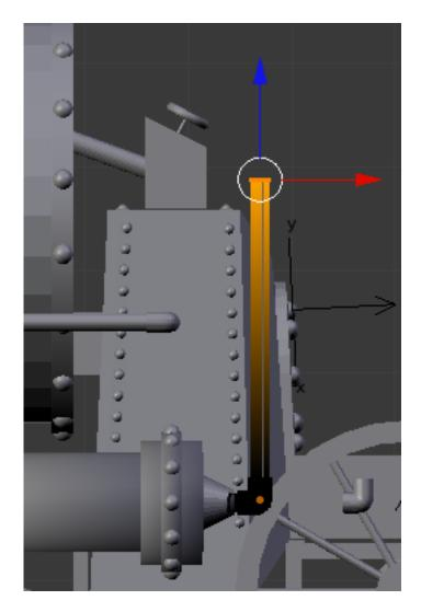
Press SHIFT-S and snap your cursor to the selected. TAB out of edit mode and select one of the duplicate pipe fittings. Press SHIFT-S and snap the fitting to the cursor.
