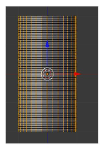
TAB out of edit mode. Press SHIFT-A and add a Bezier Curve object. Set the X rotation to 90 degrees.
