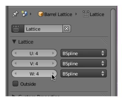
Select the Barrel object and add a Lattice modifier to it. Choose the Barrel Lattice as the Object.
