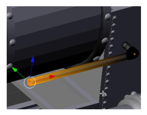
While still in edit mode and the vertices selected press SHIFT-S and snap your cursor to the selected. This will place your cursor in the center of the pipe at that end. TAB out of edit mode.
