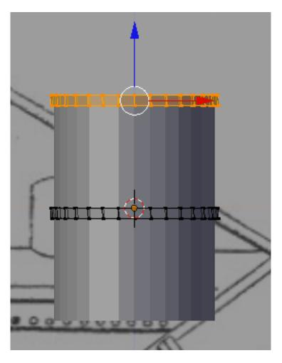
Make another copy of the vertices and move them to the bottom of the barrel. TAB out of edit mode and name this object Barrel Rings.
