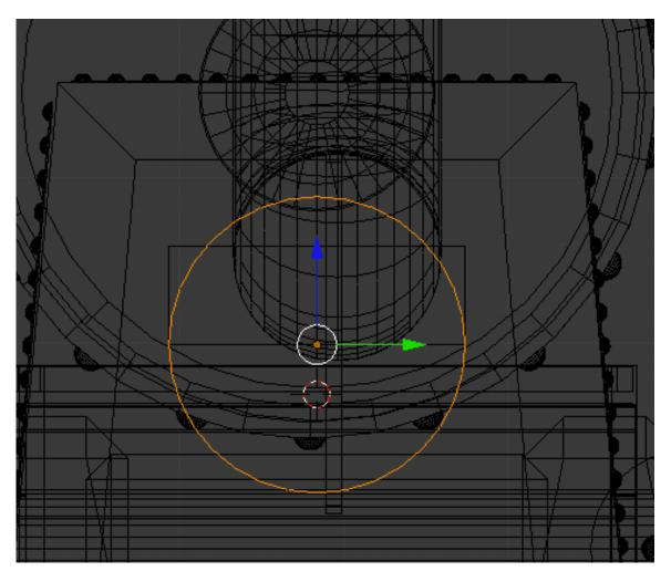
TAB into edit mode. Select the bottom vertices and delete them leaving an arc of vertices as shown below (note the middle vertices are not deleted).
