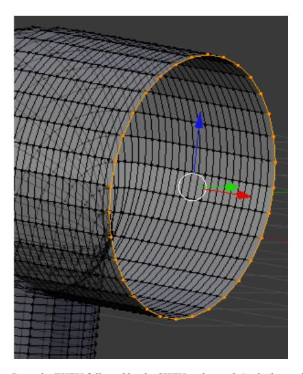
Press the EKEY followed by the SKEY and extrude/scale the vertices in a bit as shown below.
