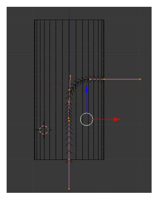
TAB out of edit mode. Select the tube object. Add a Curve modifier to it. Select the Bezier curve as the "Object".
