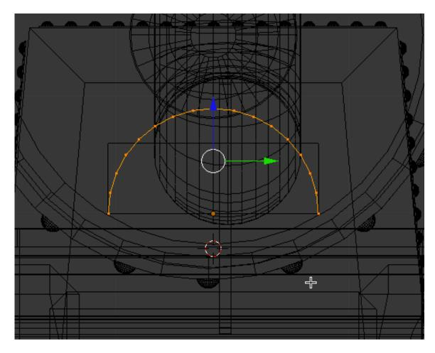
Select the 2 bottom vertices and press the EKEY (Extrude) followed by the ZKEY and extrude the vertices down as shown below.
