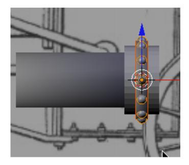
Select the tube object and name it "Piston Detail". Press the Smooth button in the 3D editor viewport tools panel to smooth the object.
