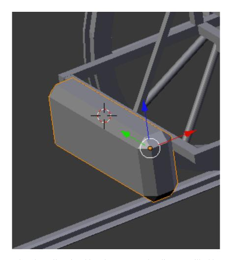
Select the Boiler Rim object that we created earlier. We will add a series of rivets to this object as well. With the Boiler Rim object selected press the MKEY and place it on layer 2 to isolate it. Then go to layer 2.
