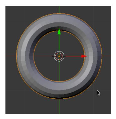
Press SHIFT-A and add a tube object. Set the X rotation to 90 and scale it down as shown below.
