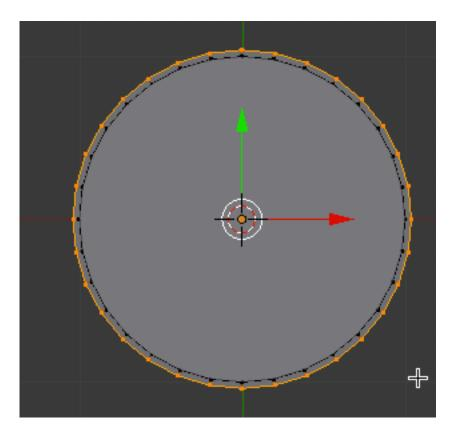
Go to front view. Select all of the vertices and extrude down along the Z-axis a bit to form a barrel ring as shown below.
