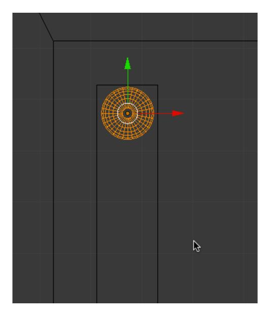
Select the Furnace Rivet and add an ARRAY modifier (this is another way to make duplicate objects.)
