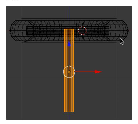
Select all of the objects and press CTRL-J and join them into one object named "Control Valve". Press the MKEY and place the control valve object on layer 1. Go to layer 1.
