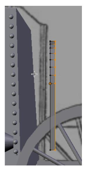
Rotate your view so you can see the door more dimensionally. We need to fill the front with faces. To make the faces cleaner, select the two vertices at the bottom of the arch as shown below and press the FKEY. This will create an edge there.
