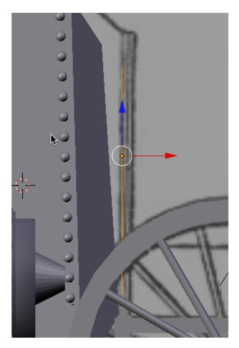
TAB into edit mode. Select all the vertices. Extrude them out a bit along the X-axis as shown below.
