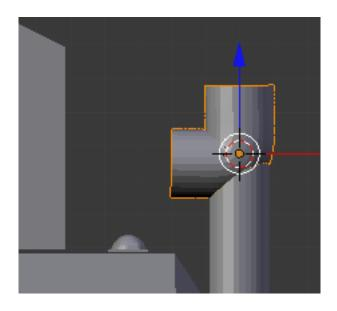
Rotate the fitting 180 degrees around the X-axis. TAB into edit mode. Select the inner ring of vertices and extrude them out along the X-axis as shown below.
