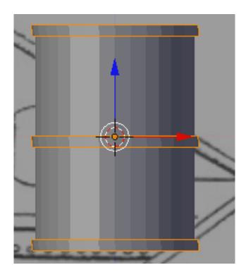
Select the tube object. TAB into edit mode. Press CTRL-TAB and go to edge select mode. Box select the inside edges. Press the Subdivide button in the 3D editor tool panel 5 times. (We need lots of vertices to perform the next deform operation)
