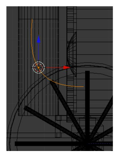
Select the separated object. Add a Curve modifier to the object. Click on the Object box and select the Stack Curve as the object.
