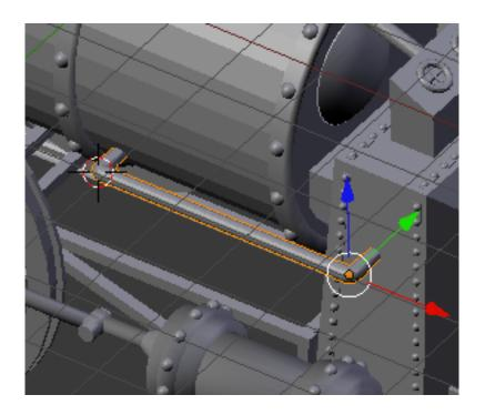
Make a duplicate copy of the Pipe 1 object and move it to the other side of the engine. Rotate it 180 degrees about the X-axis and position it. Name the duplicate object Pipe 2.
