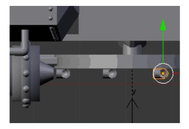
Select the first fitting and extrude one set of inside vertices along the X-axis into the piston and extrude the other set of vertices up along the Z-axis as shown below.
