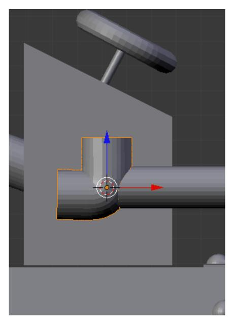
Rotate the fitting 90 degrees around the Y-axis and the rotate it -90 degrees around the X-axis.
