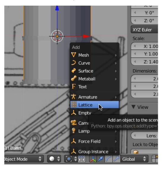
A Lattice is a cage like object that we will use to deform the barrel shape.
