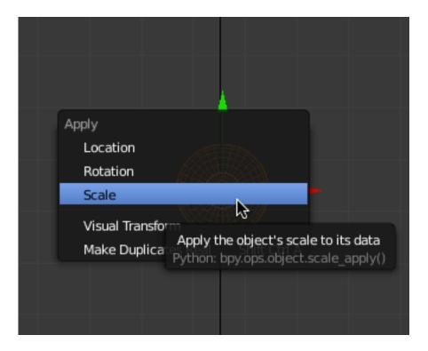
This will reset the scale of the object. Note the scale in the properties panel now reads "1".
