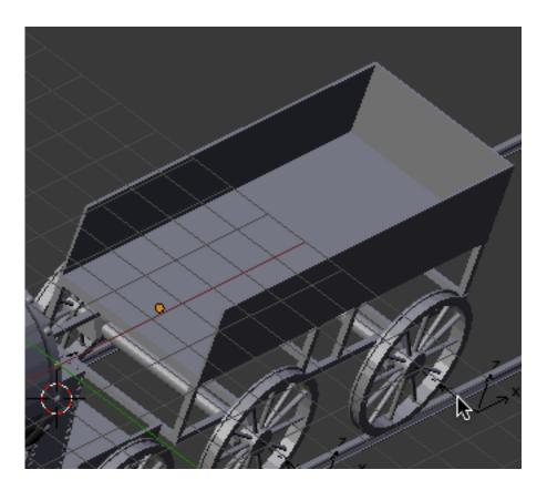
We will put some rivet trim on the car as well. Go to top view. Select the Furnace Rivet and Rivet plate objects from the top of the furnace. Press SHIFT-D and move the duplicate objects along the X-axis to the rear of the car as shown below.
