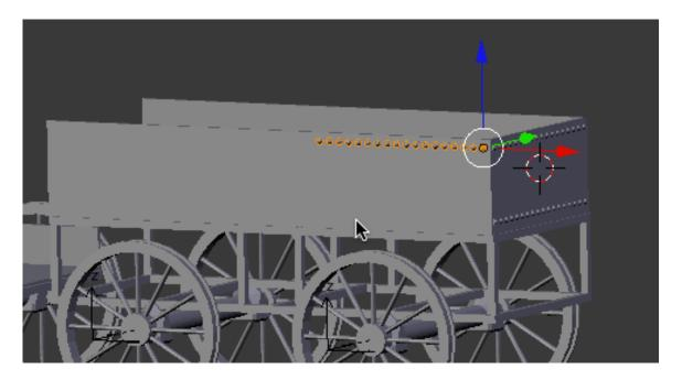
Edit the plate object to extend it the length of the side of the car and then increase the count of the rivet array modifier to fill up the space with rivets (mine took 46).
