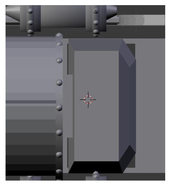
Go to wireframe display mode and press SHIFT-A and add a plane object. Edit the plane as shown below. Set the origin to the geometry (SHIFT-CTRL-ALT-C).
