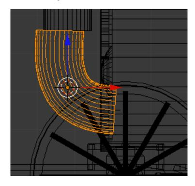
The curve of the separated object is controlled by the location and shape of the Stack Curve object. We can select the target stack curve object and TAB into edit mode and alter the curve and the separated object will reflect those edits.
