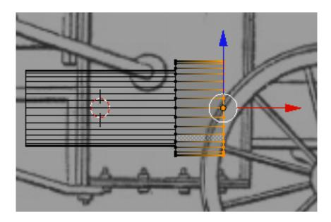
Deselect the vertices and TAB out of edit mode. Go to layer 1. Select both the stack collar and collar rivet objects (located at the top of the smoke stack). Press SHIFT-D and make a duplicate copy of these two objects and move them to the side of the stack as shown below.
