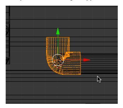
Rotate and zoom your view so you can see the side of the fitting facing the boiler. TAB into edit mode and select the inner ring of vertices and extrude them along the Y-axis into the boiler object as shown below.
