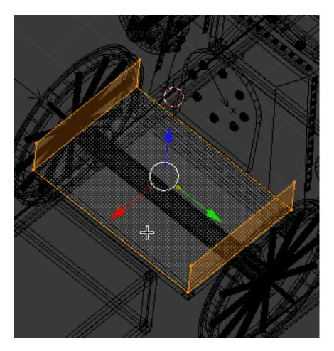
Tab out of edit mode. Add a SOLIDIFY modifier to the object. Set the thickness to .08 This modifier adds thickness to the faces of an object.
