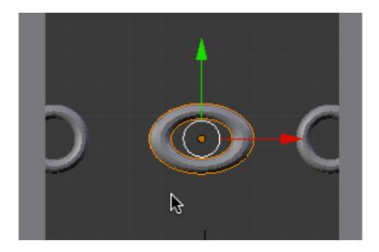
Press SHIFT-D, then press the RKEY followed by the XKEY followed by 90 then ENTER. This will make a duplicate and rotate it 90 degrees around the X-axis. Move this object to the left as shown below.
