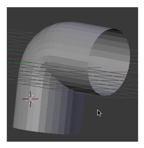
Select the pipe fitting object and TAB into edit mode. Press CTRL-TAB and go to vertex select mode. Hold your ALT KEY down and select one of the vertices on the edge of the fitting. This will select the whole loop of vertices.
