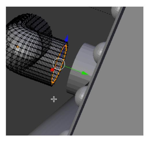
Press the EKEY and extrude the vertices along the Y-axis into the furnace as shown below.
