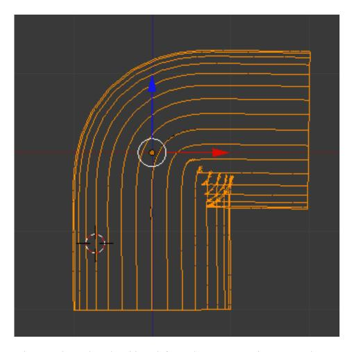
When you have the tube object deformed, as you want it, APPLY the curve modifier. Once the curve modifier has been applied you can delete the Bezier curve object.
