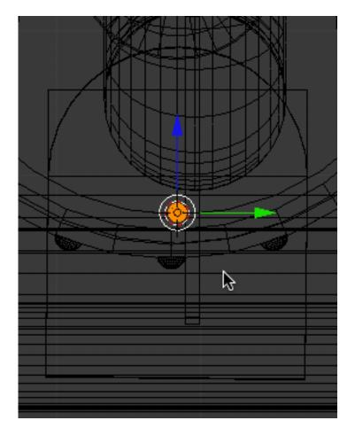
Press the MKEY and place this object on layer 2 so we can work on it easier. Go to layer 2.
