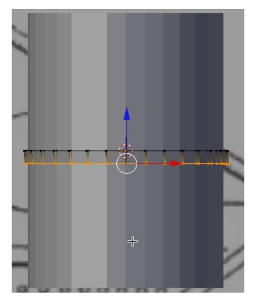
Select all of the vertices then press SHIFT-D, then press the ZKEY and make a duplicate of the vertices and move them to the top of the barrel.
